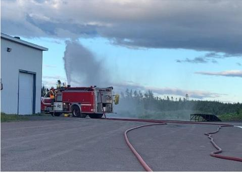
**Photo 7.** Relay Pumping with Master Streams Training.
