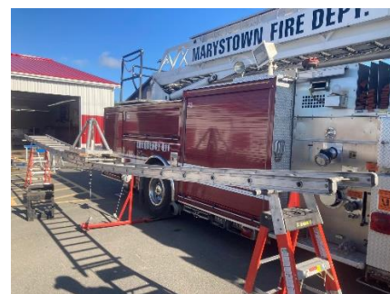
Photo 4. Annual Ground Ladder testing.
