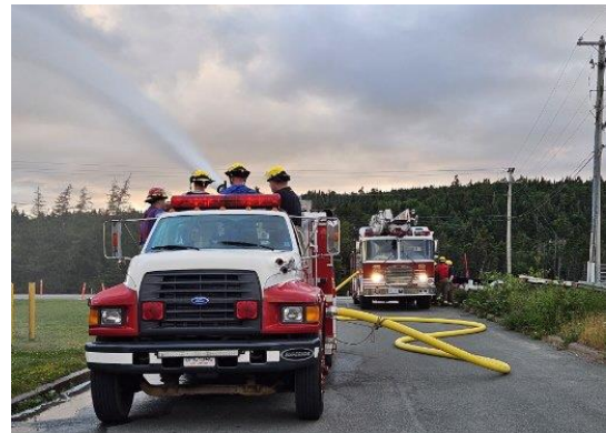
Photo 20. Pump Operations training with Relay Pumping.
